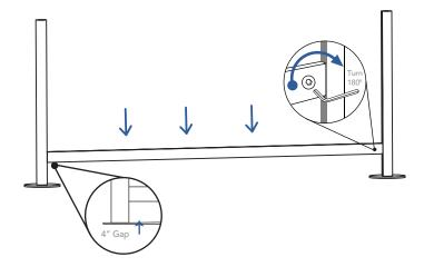
Finish securing the frame, by locking the last horizontal bar into the post channel.
