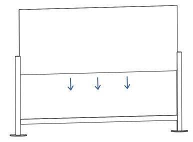
Leaving a 4" gap above the bases, attach the horizontal bar by locking it into the post channel.
