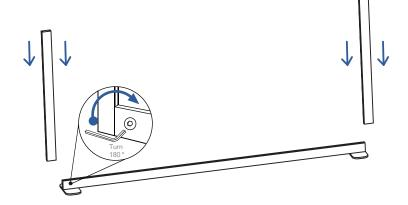
The system should be assembled. If the acrylic panel is resting on the bottom horizontal bar, remove the panel and insert a spacer into each vertical channel.
