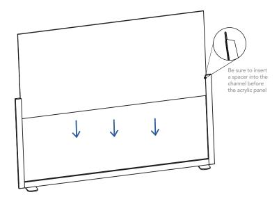
Attach the vertical posts by locking them into horizontal bar's top channel.
